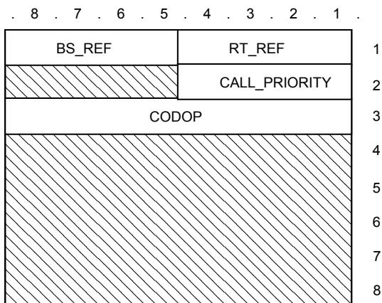
Figure 31: D\_DCH\_OPEN TSDU format
