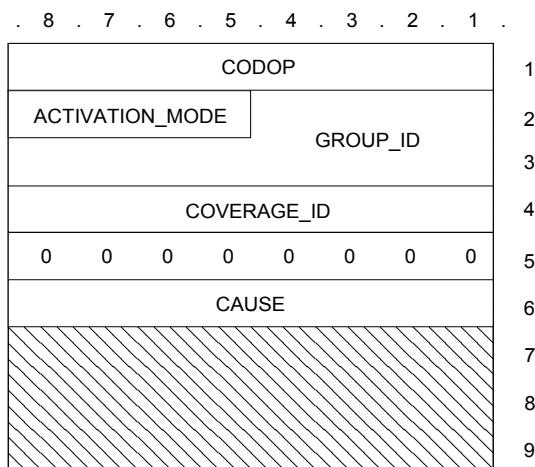
Figure 54: D\_GROUP\_REJECT TSDU format
