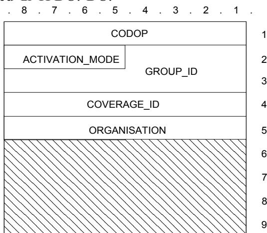
Figure 52: D\_GROUP\_OVERLOAD\_ID TSDU format
