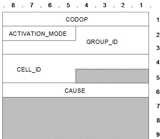
Figure 37: D\_ECH\_REJECT TSDU format
