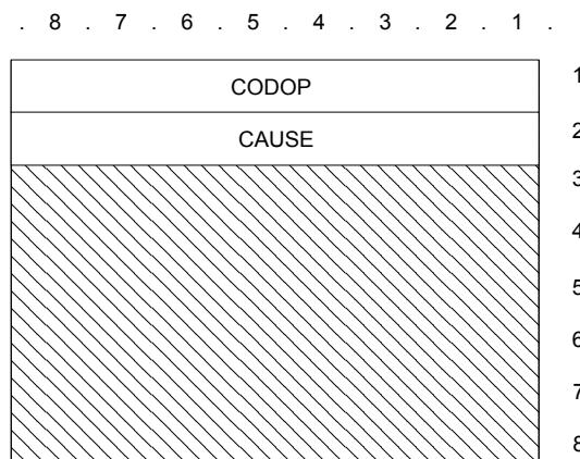
Figure 26: D\_DATA\_END TSDU format
