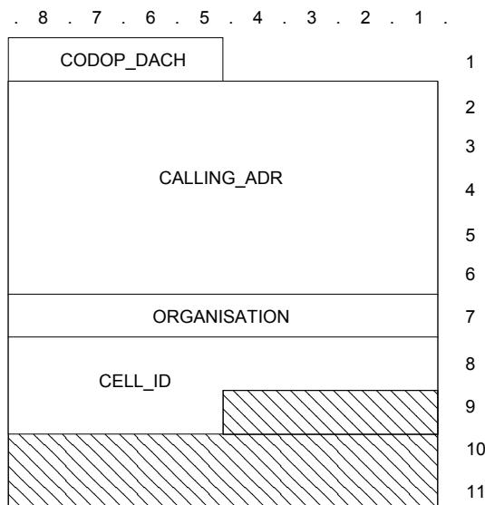
Figure 113: U\_EMERGENCY\_ACK TSDU format
