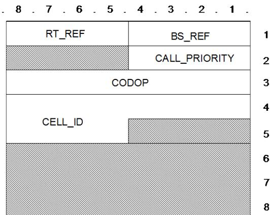
Figure 96: U\_CALL\_INTRUSION\_ECH TSDU format
