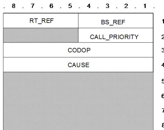
Figure 131: U\_TERMINATE TSDU format
