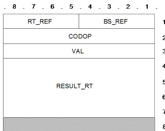
Figure 102: U\_CALL\_SWITCH TSDU format
