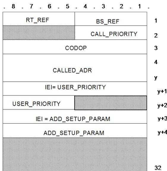
Figure 101: U\_CALL\_SETUP TSDU format
