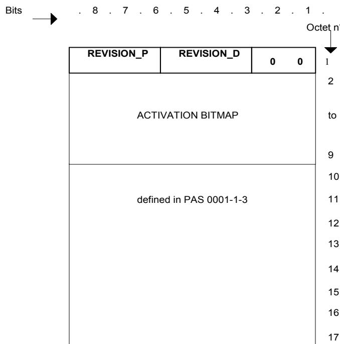
**Figure 65: D\_PCH TSDU format**
