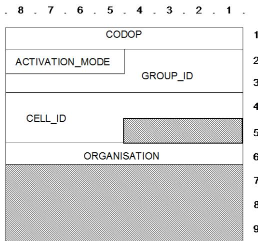
Figure 36: D\_ECH\_OVERLOAD\_ID TSDU format
