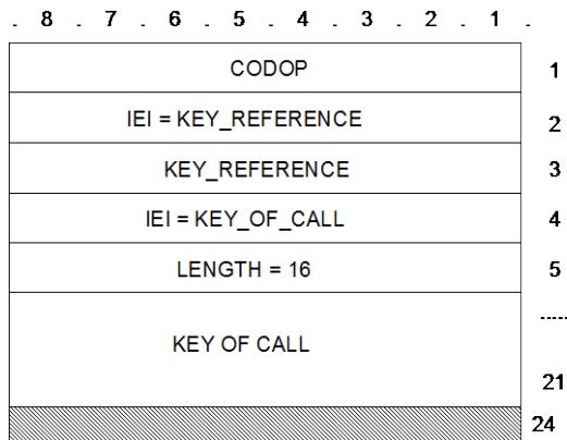
**Figure 16: D\_CALL\_START TSDU format**
