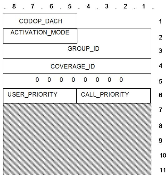
Figure 129: U\_OC\_ACTIVATION TSDU format
