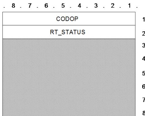
Figure 60: D\_LOCATION\_ACTIVITY\_ACK TSDU format
