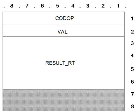
Figure 91: U\_AUTHENTICATION TSDU format
