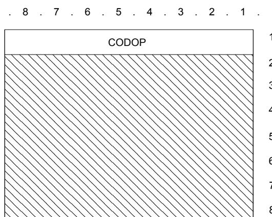
Figure 38: D\_EMERGENCY\_ACK TSDU format
