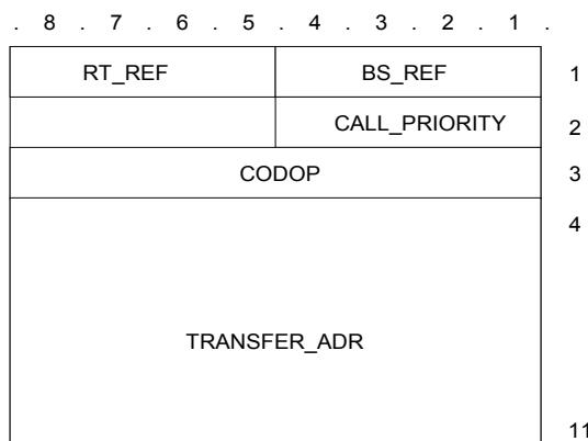
Figure 133: U\_TRANSFER\_REQ TSDU format
