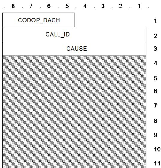
Figure 99: U\_CALL\_REJECTED TSDU format
