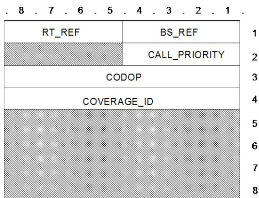
Figure 124: U\_OCH\_RELEASE TSDU format
