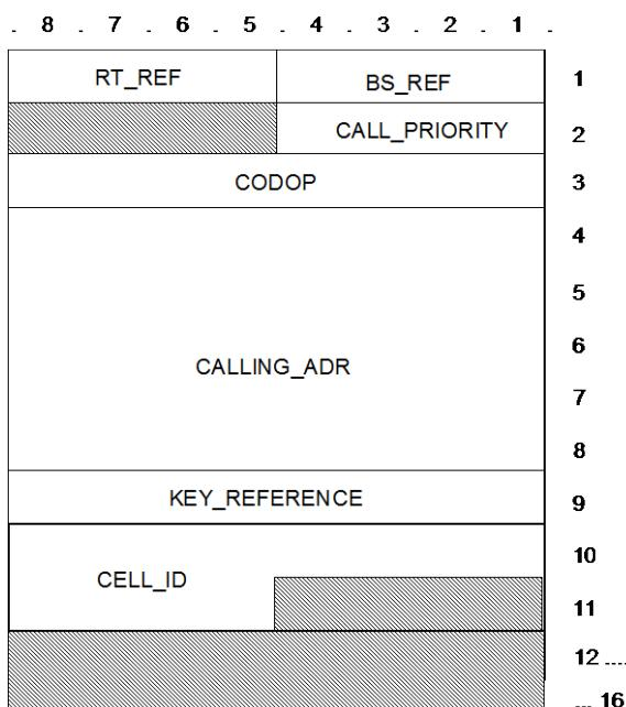
Figure 112: U\_ECH\_SETUP TSDU format
