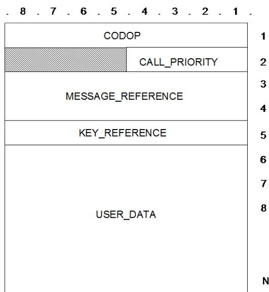
Figure 10: D\_BROADCAST TSDU format
