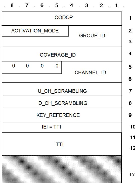
Figure 46: D\_GROUP\_ACTIVATION TSDU format
