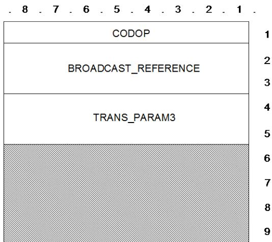
Figure 12: D\_BROADCAST\_WAITING TSDU format
