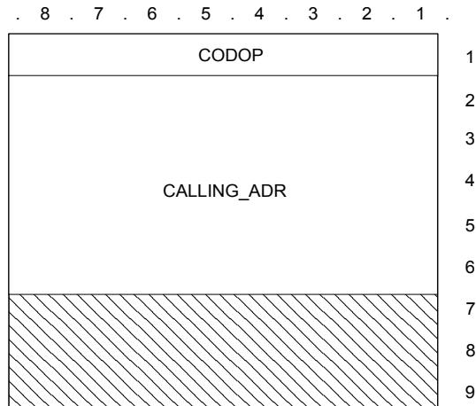
Figure 44: D\_FORCED\_REGISTRATION TSDU format
