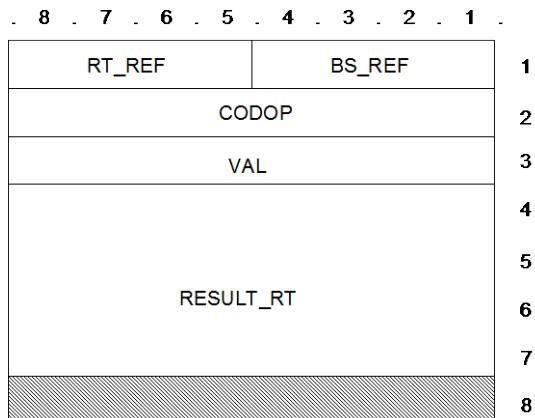
Figure 104: U\_DATA\_DOWN\_ACCEPT TSDU format
