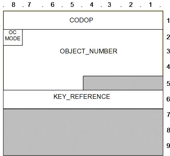
Figure 63: D\_OC\_PAGING TSDU format
