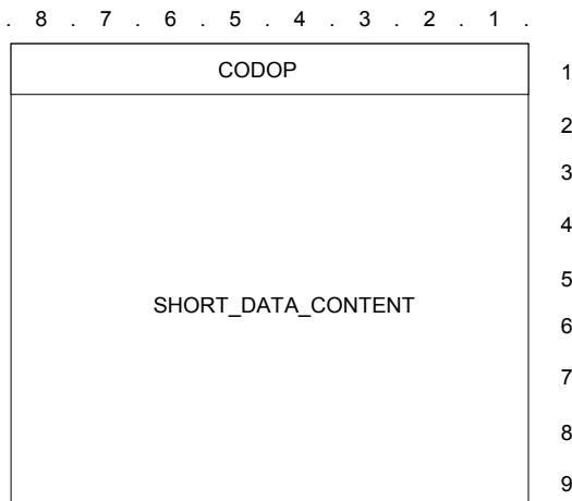
**Figure 45: D\_FUNCTIONAL\_SHORT\_DATA TSDU format**
