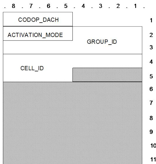
Figure 110: U\_ECH\_ACTIVATION TSDU format
