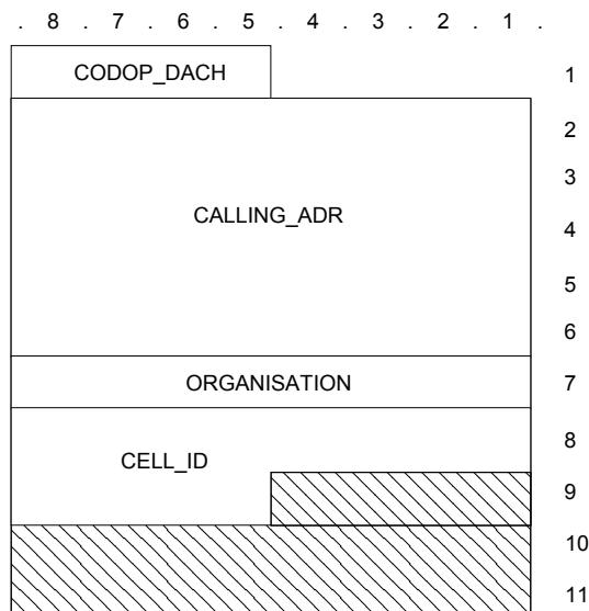
Figure 114: U\_EMERGENCY\_NAK TSDU format
