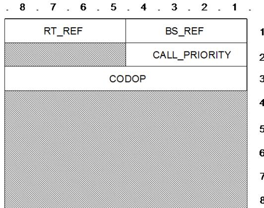
Figure 108: U\_DEVIATION\_CLEAR TSDU format
