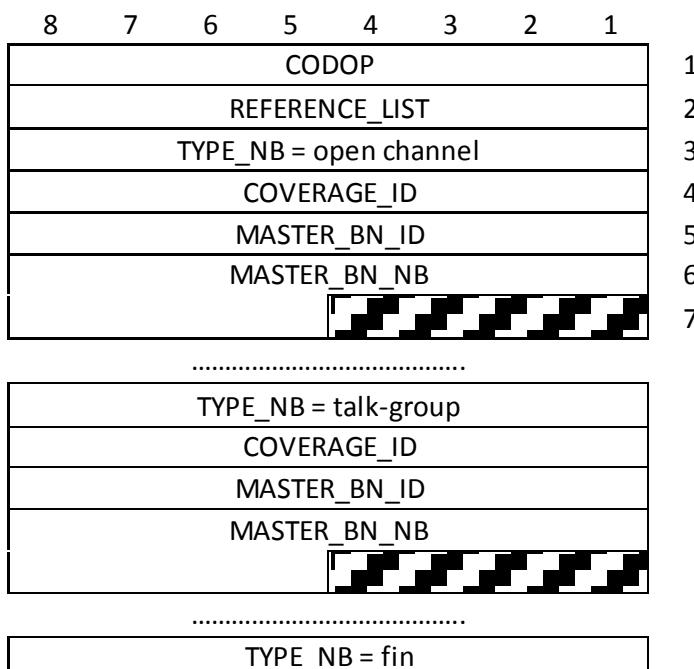
Figure 51: D\_GROUP\_MASTER TSDU format
