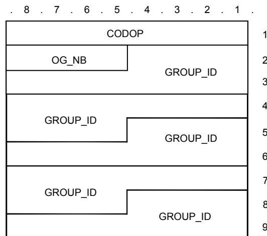
Figure 11: D\_BROADCAST\_NOTIFICATION TSDU format
