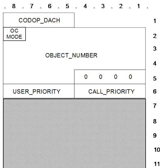
Figure 123: U\_OC\_ACTIVATION TSDU format
