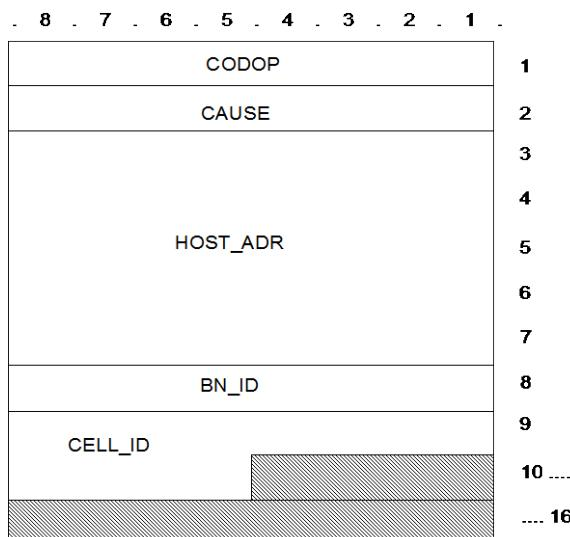
Figure 72: D\_REGISTRATION\_NAK TSDU format
