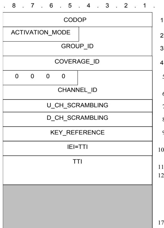
Figure 68: D\_PRIORITY\_GRP\_ACTIVATION TSDU format
