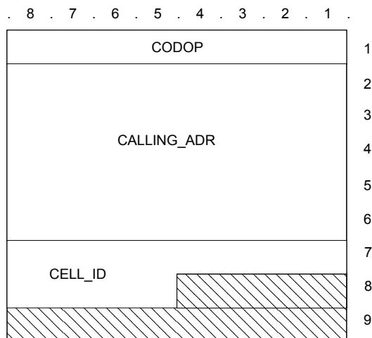
Figure 40: D\_EMERGENCY\_NOTIFICATION TSDU format
