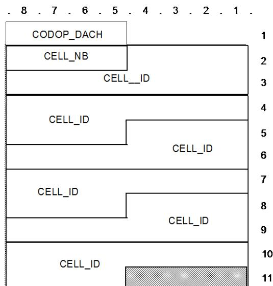
Figure 128: U\_PRIORITY\_GRP\_WAITING TSDU format
