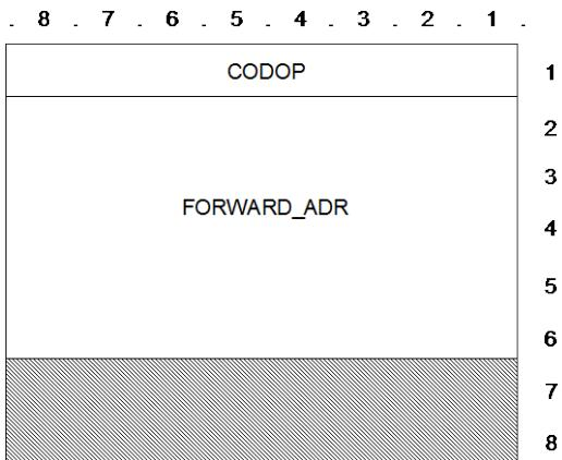
**Figure 33: D\_DEVIATION\_ON TSDU format**
