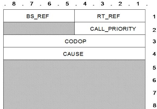
Figure 74: D\_RELEASE TSDU format
