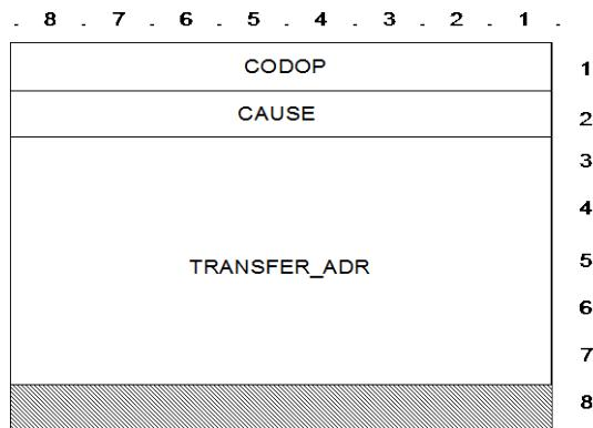
Figure 85: D\_TRANSFER\_NAK TSDU format
