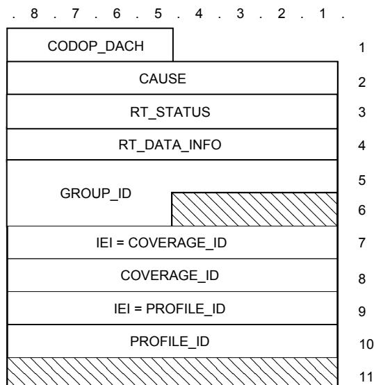
Figure 90: U\_ATTACH TSDU format
