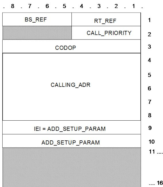
**Figure 15: D\_CALL\_SETUP TSDU format**
