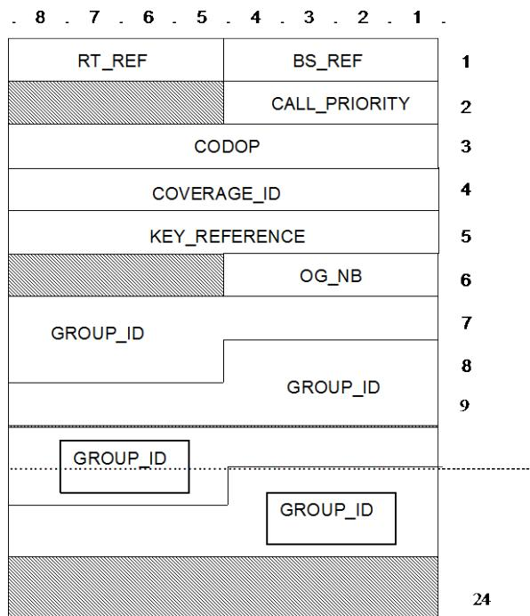
Figure 125: U\_OCH\_SETUP TSDU format
