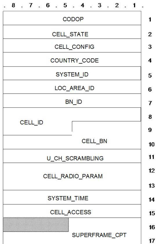
Figure 78: D\_SYSTEM\_INFO TSDU format
