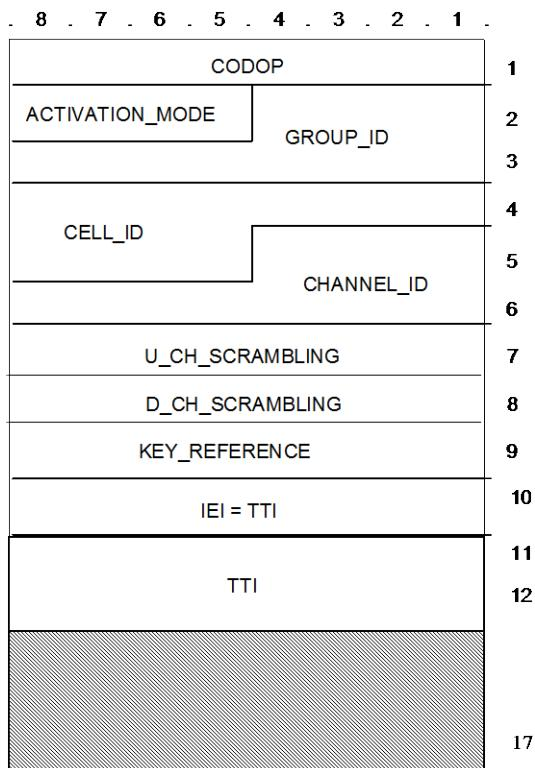
Figure 35: D\_ECH\_ACTIVATION TSDU format
