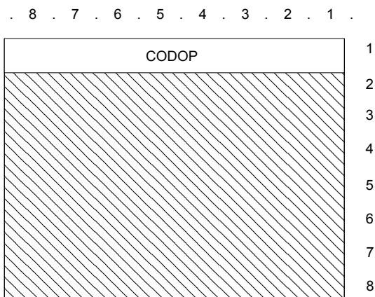
Figure 41: D\_END or U\_END TSDU format
