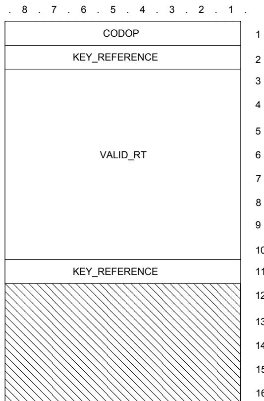
Figure 24: D\_DATA\_AUTHENTICATION TSDU format
