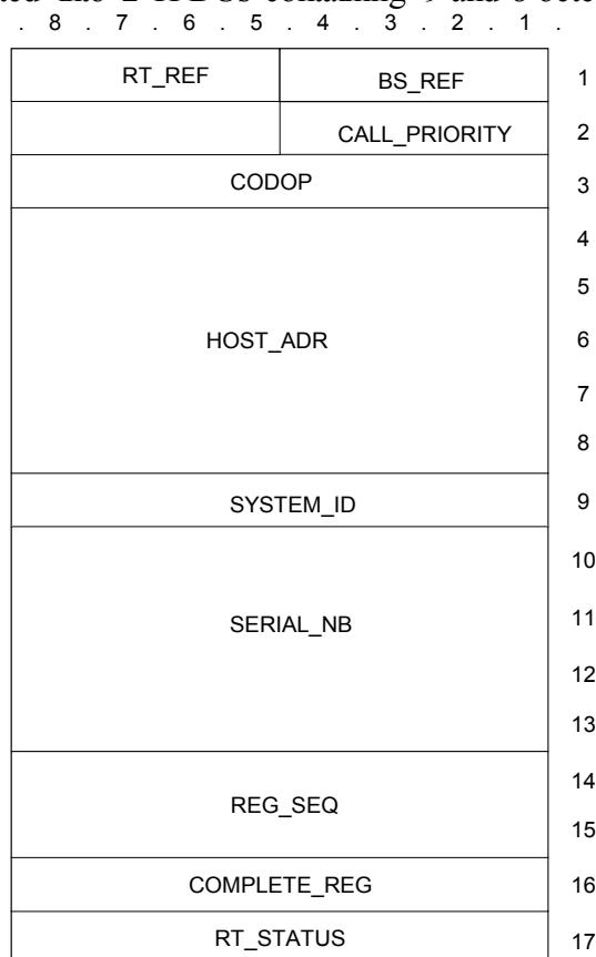
Figure 127: U\_REGISTRATION\_REQ TSDU format
