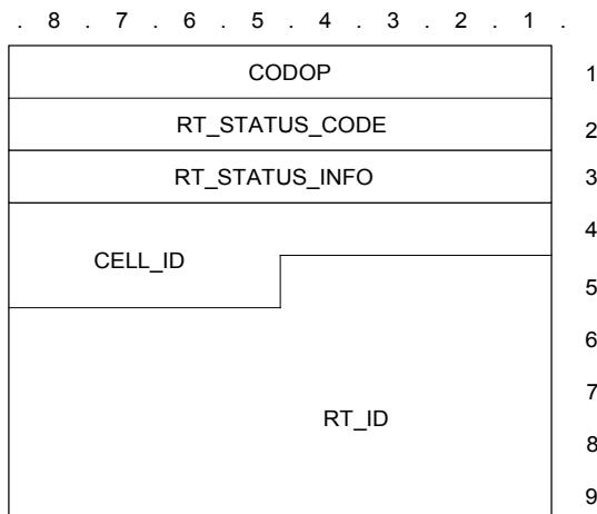
Figure 25: D\_DATA\_DOWN\_STATUS TSDU format
