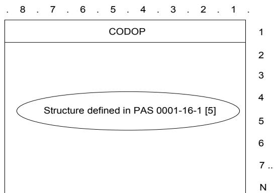
Figure 58: D\_KEY\_END\_DELIVERY TSDU format
