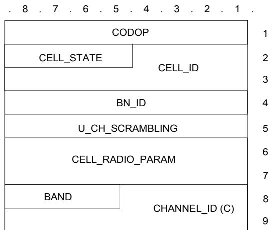
Figure 79: D\_SYSTEM\_INFO TSDU format in BSC-disconnected mode
