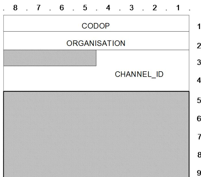
Figure 20: D\_CHANNEL\_INIT TSDU format
