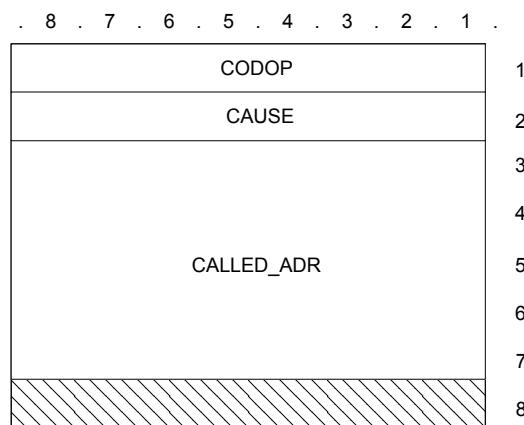
**Figure 9: D\_BACK\_CCH TSDU format**
