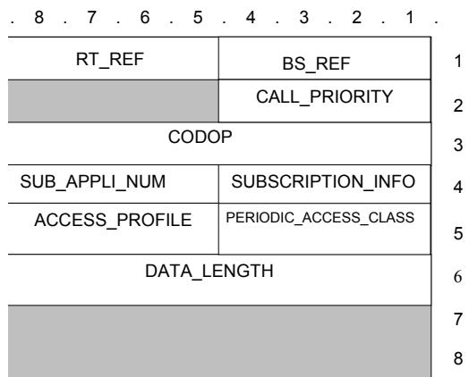
Figure 126: U\_PERIODIC\_ACCESS\_SUBSCRIPTION\_RQ TSDU format
