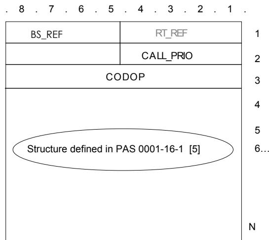
**Figure 3: D\_ABILITY\_MNGT TSDU format**
