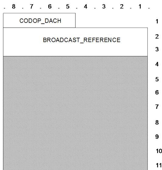
Figure 92: U\_BROADCAST\_ACCEPTED TSDU format
