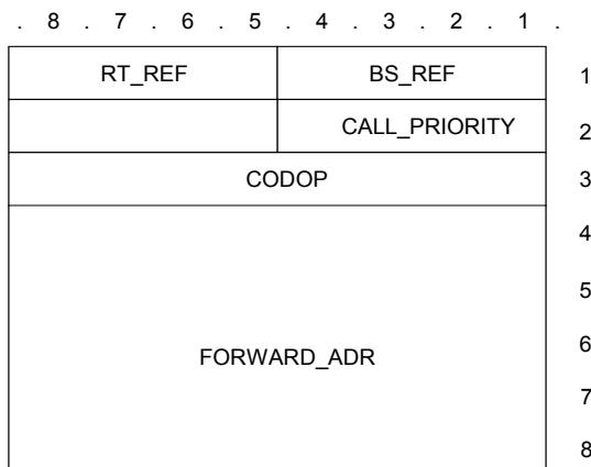
Figure 109: U\_DEVIATION\_SET TSDU format
