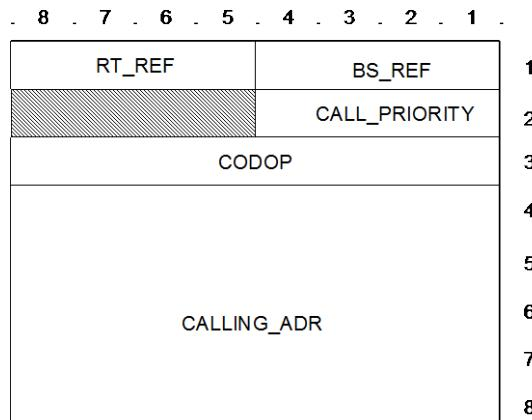
Figure 98: U\_CALL\_INTRUSION\_PC TSDU format
