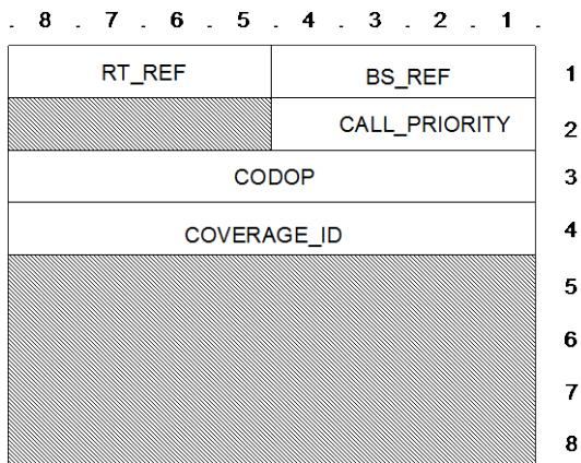
Figure 97: U\_CALL\_INTRUSION\_OCH TSDU format
