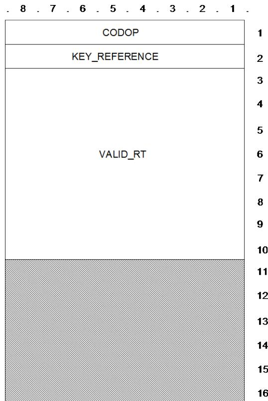
Figure 7: D\_AUTHENTICATION TSDU format
