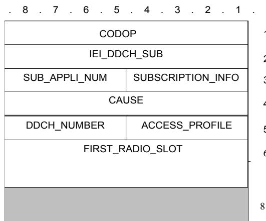
Figure 66: D\_PERIODIC\_ACCESS\_SUBSCRIPTION\_ACK TSDU format
