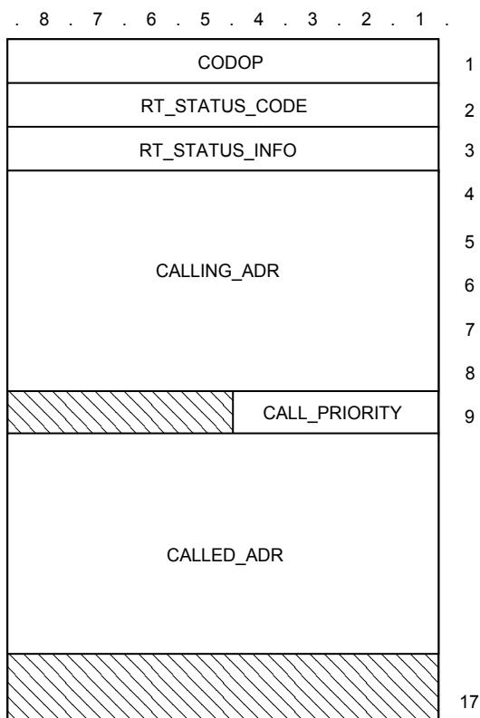
Figure 43: D\_EXTENDED\_STATUS TSDU format
