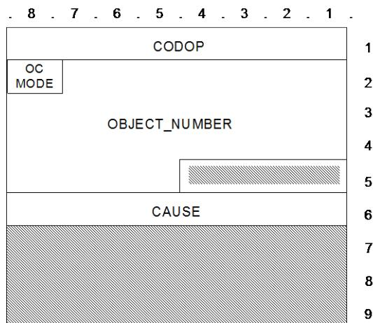
Figure 64: D\_OC\_REJECT TSDU format
