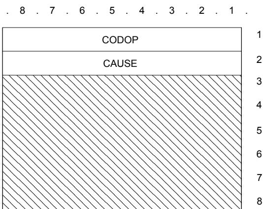
Figure 39: D\_EMERGENCY\_ACK TSDU format
