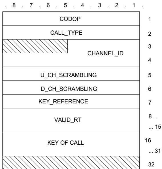
Figure 14: D\_CALL\_CONNECT TSDU format
