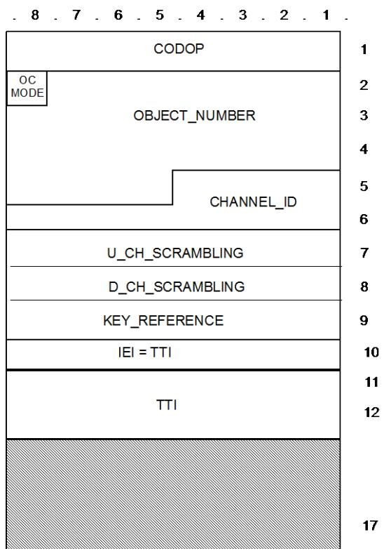
Figure 62: D\_OC\_ACTIVATION TSDU format
